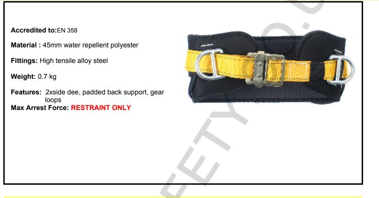
The RGB2 is essentially an RGB1 with alternative buckle and gear loops fitted, and is a work positioning / restraint belt (see the info sheet on restraint vs. fall arrest). This belt is fitted with two side mounted dee rings for ease of attachment and the back pad provides some lumber support and comfort, especially when tools are hung from the belt loops.
