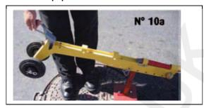
**b. Detaching magnet in an easier way:** using handle-bar shaft in retracted position. To separate magnet from plate, put handle-bar shaft in retracted position, and use LIFTPAQ® lifting handle or body to pull up until magnet detaches itself. During this operation, the handle-bars are pushed against the ground.
