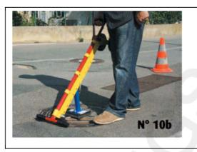
b. Detaching magnet in an easier way: using retracted handle. To separate magnet from plate, pull handle back fully, use LIFTPAQ lifting handle or body to pull up until the magnet is detached. During this operation, instrument handles will be pushing on the ground.
