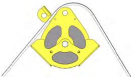
1. Remove the axis, shift the brace and install the cable.
