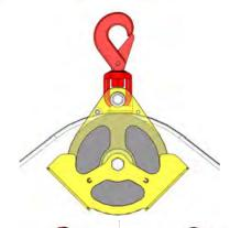
2. Put the brace back in place; place the axis (and the hook if the pulley is equipped with a hook).
