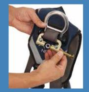
Slide connector through loosened web straps below back D-ring, then pull straps tight.
